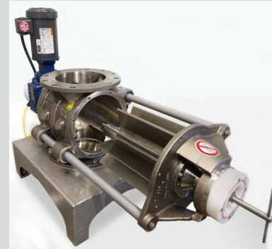
3. Slide out endplate and rotor.
