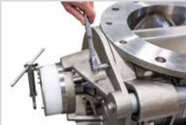
1. Remove endplate fasteners.
