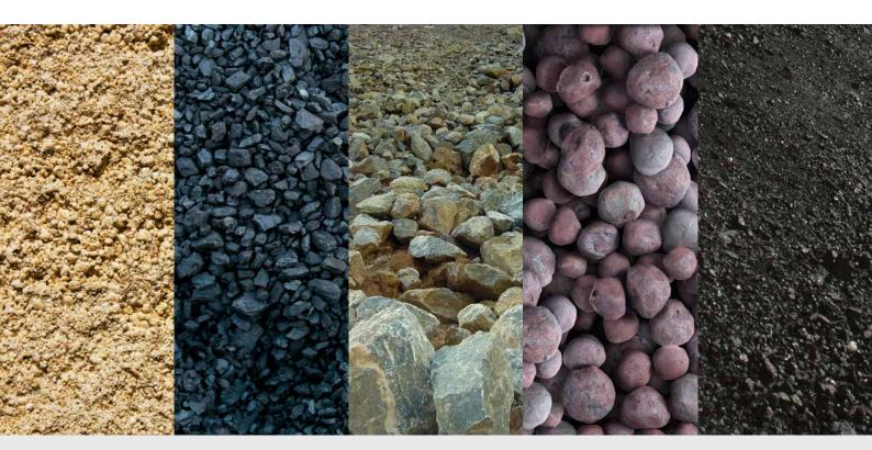
Schenck Process has an extensive materials database covering over 10,000 samples for which characteristics such as particle size distribution, shape, porosity, bulk density, temperature, moisture content, fragility and air retentiveness have been measured and the most suitable conveying method determined.
