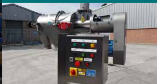
Kek K300C Sifter with Integral Control Panel
