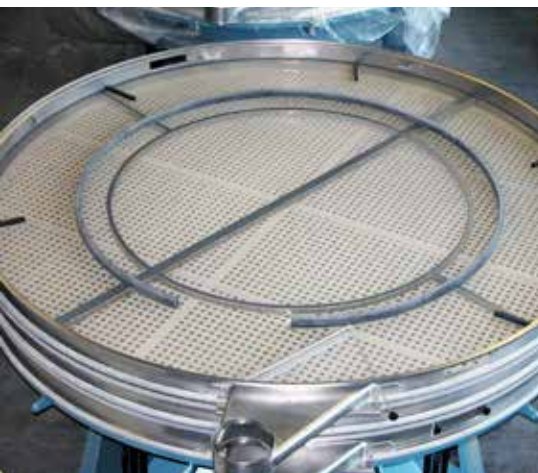
View of Tumbler Screener, Screen Deck
