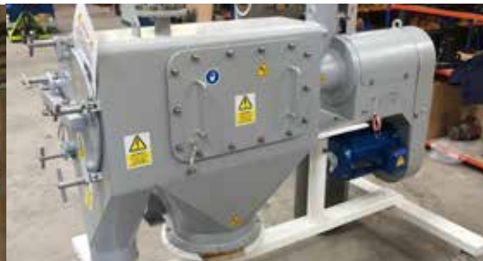
Kek K650CP In-Line Pressure Sifter with Bolted Side Door
